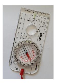
First we need to turn at a right angle to our bearing. In the above example, our bearing is 220 degrees. The easiest way to do this without adjusting the bearing is by turning the whole compass so the North-South magnetic needle aligns with the East - West markings on the compass housing. See below:
