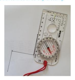
Again, once we are clear of the obstacle, we then turn our bearing 90 degrees using the same method as before. This time in the opposite direction to the first 90 degrees.
