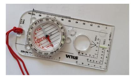
Once we have turned our bearing by 90 degrees, the direction of travel arrow now points us in the direction we need to walk in. We measure the distance along this bearing, using pacing, until we are clear of the obstacle.
