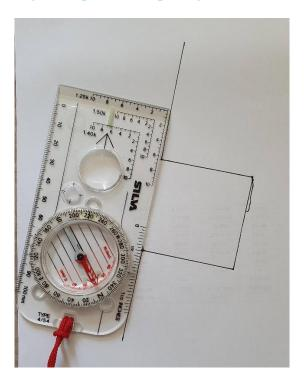
If you are pacing or timing a distance and you come across an obstacle that you need to box around, you must only add the distance for the side of the box that is parallel to your original bearing, to your total distance. The distances paced on the detours do not count towards your total distance and/or time of your leg. Remember to stop a stopwatch on the detours and restart it when walking only on your original bearing.
